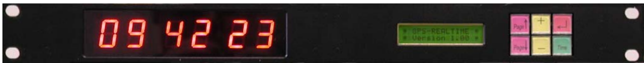
Fig.1 1RU 19" GPS LTC Time Code Real Time Central Unit GPSLTCRTC119
